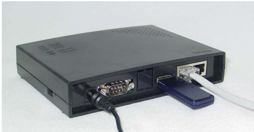
<Fig. 1.3> Parani-MSP100 attached with USB extension dongle
