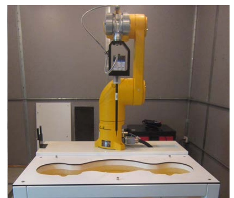
Figure 4.1 DASY5 Test System
