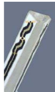
Figure 3.3 Probe Thick-Film Technique
