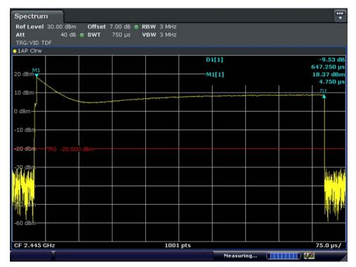
Note DCCF(Duty Cyle Correction Factor) :  $20\log_{10}($  Pulse width / Period of the pulse train ) =  $20\log_{10}($  (1 × 0.647ms) / 100 ms ) = -43.78 dBm
