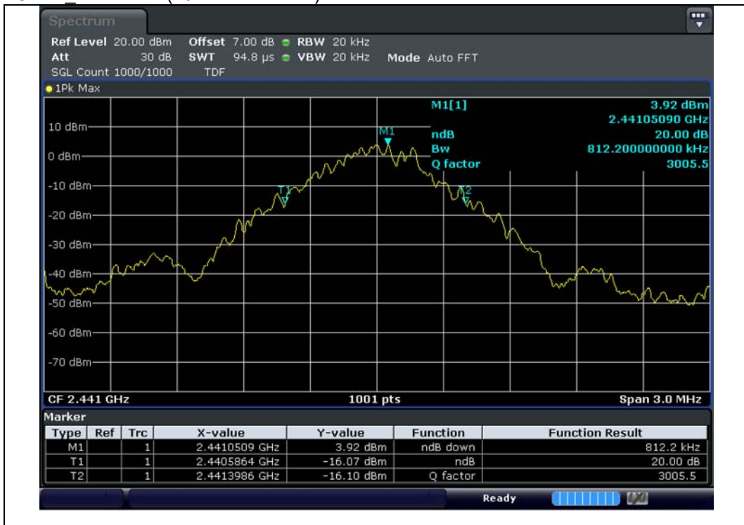
GFSK 2 441 MHz(20 dB Bandwidth)
