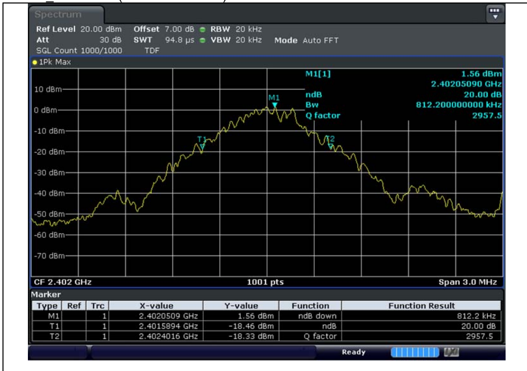
GFSK 2 402 MHz(20 dB Bandwidth)
