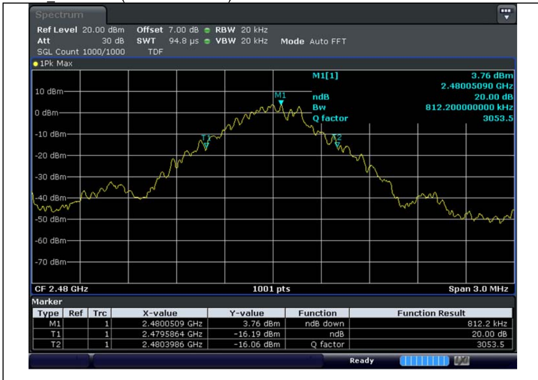
GFSK 2 480 MHz(20 dB Bandwidth)
