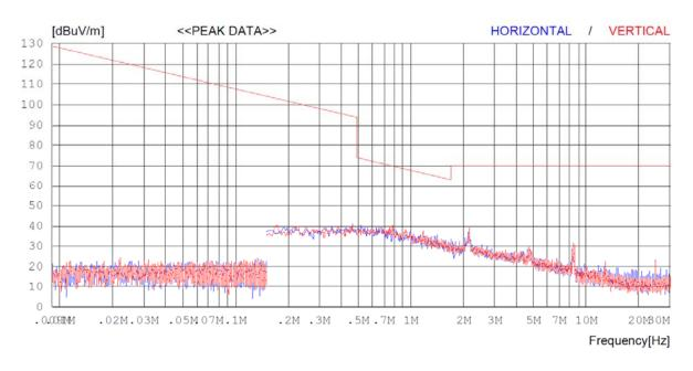
Test mode : 9 kHz ~ 30 MHz ( Worst case : Zigbee / Highest Frequency)
