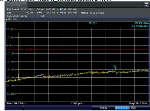
Test mode : Zigbee / Middle Frequency Conducted Spurious Emission
