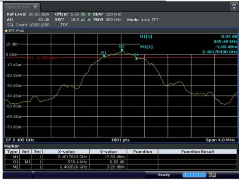
Test mode: MASTER Bluetooth LE / 2 440 MHz 6 dB Bandwidth
