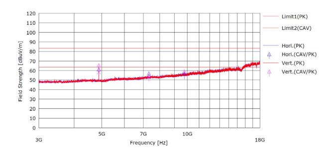
Note 1: Measured distance: 1 m Note 2: Limit: Peak: 83.5 dBµV/m Average: 63.5 dBµV/m
