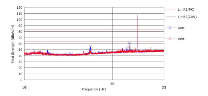
$\begin{array}{lll} \mbox{Note 1:} & \mbox{Measured distance: 1 m} \\ \mbox{Note 2:} & \mbox{Limit: Peak: 83.5 dB} \mu\mbox{V/m} \\ & \mbox{Average: 63.5 dB} \mu\mbox{V/m} \\ \end{array}$
