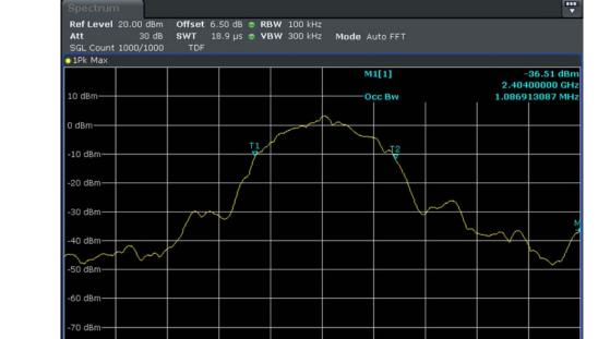
Test mode: MASTER Bluetooth LE / 2 402 MHz Occupied Bandwidth
