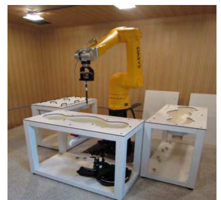
Figure 4.1 DASY5 Test System
