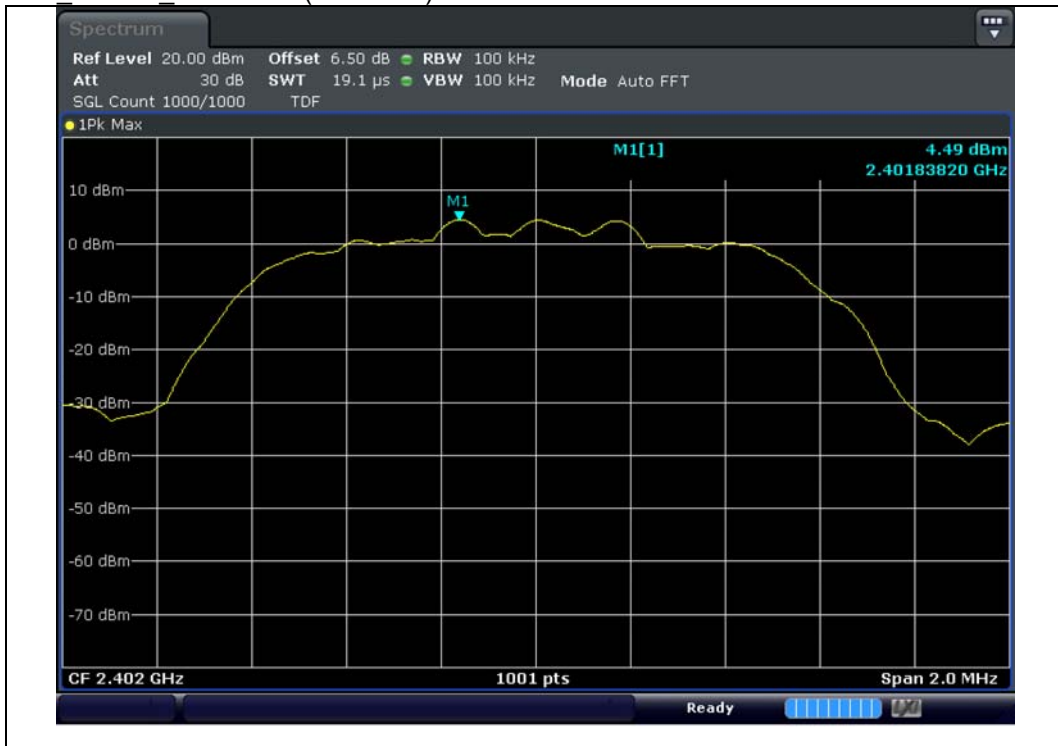
M0 8DPSK 2 402 MHz(reference)
