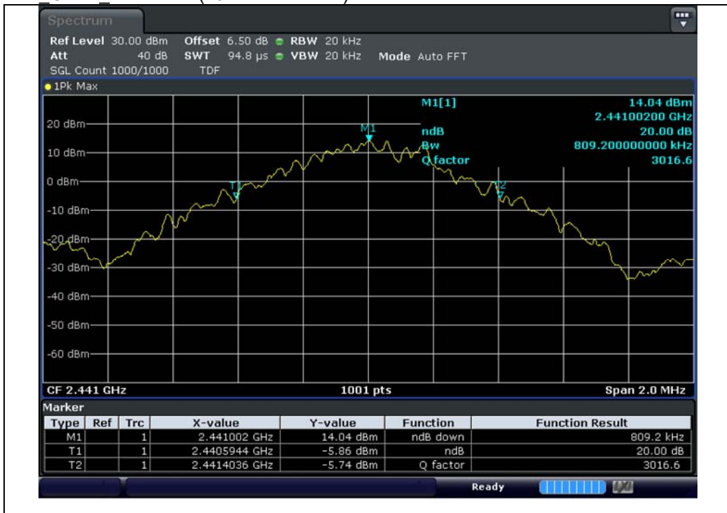
M1_GFSK_2_441_MHz(20 dB Bandwidth)
