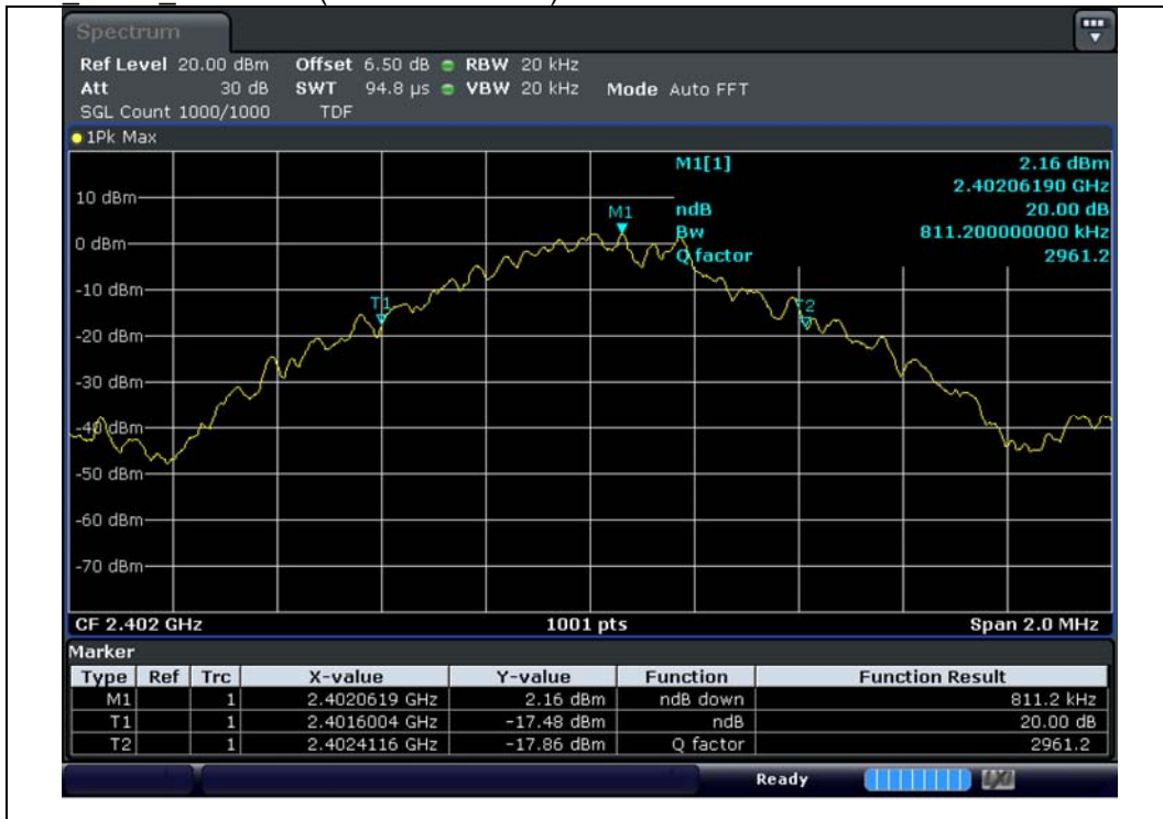
M0_GFSK_2 402 MHz(20 dB Bandwidth)
