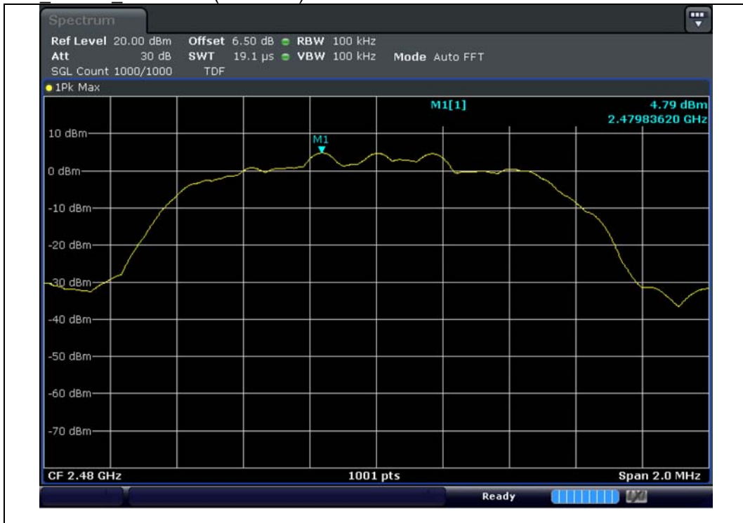
M0 8DPSK 2 480 MHz(reference)
