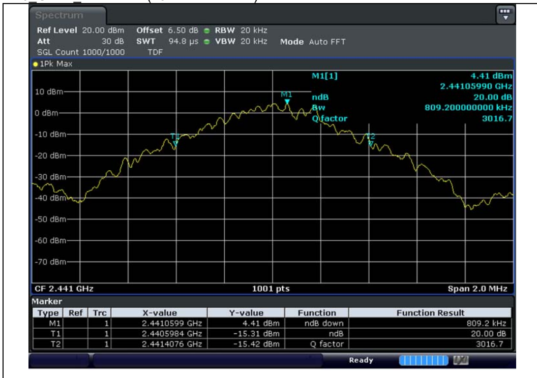
M0_GFSK_2 441 MHz(20 dB Bandwidth)
