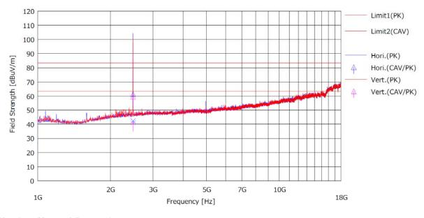
Test mode : 1 GHz ~ 18 GHz (Worst case : Bluetooth LE / Highest Frequency)
