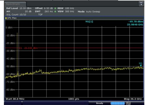
Test mode : Bluetooth LE / Lowest Frequency Conducted Spurious Emission
