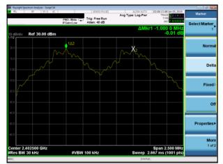
(1Mbps) Channel Separation plot on channel 39-40
