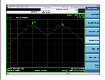
(1Mbps) Channel Separation plot on channel 77-78
