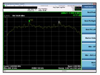
(2Mbps) Channel Separation plot on channel 39-40
