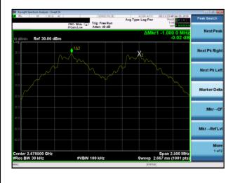
(2Mbps) Channel Separation plot on channel 00-01
