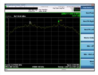
(3Mbps) Channel Separation plot on channel 77-78
