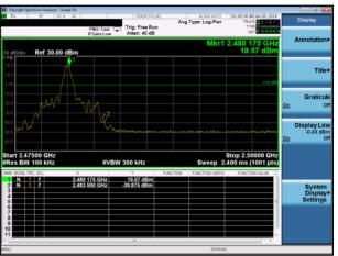
GFSK: Band Edge-High Channel (Hopping Mode)
