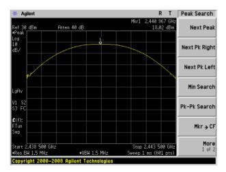
Peak output Power plot on channel 78 (1Mbps)
