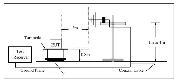
(c) For radiated emissions above 1000MHz
