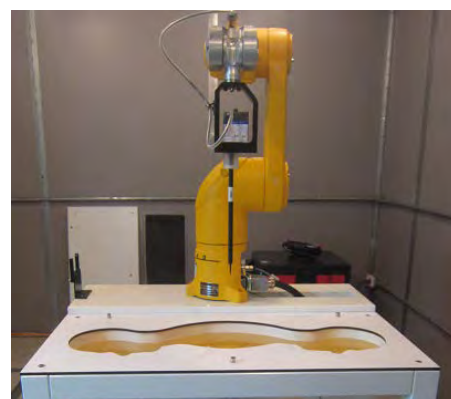
Figure 4.1 DASY5 Test System
