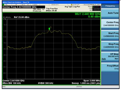
Conducted Spurious Emissions <u>Middle Channel & Modulation : 8DPSK</u>
