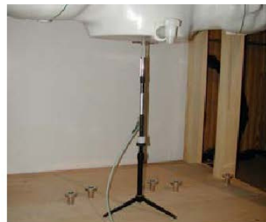
Figure 9.1 Dipole Verification Test Setup Diagram & Photo
