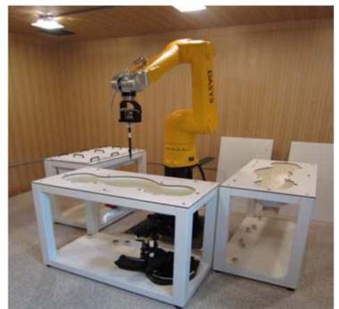
Figure 4.1 DASY5 Test System
