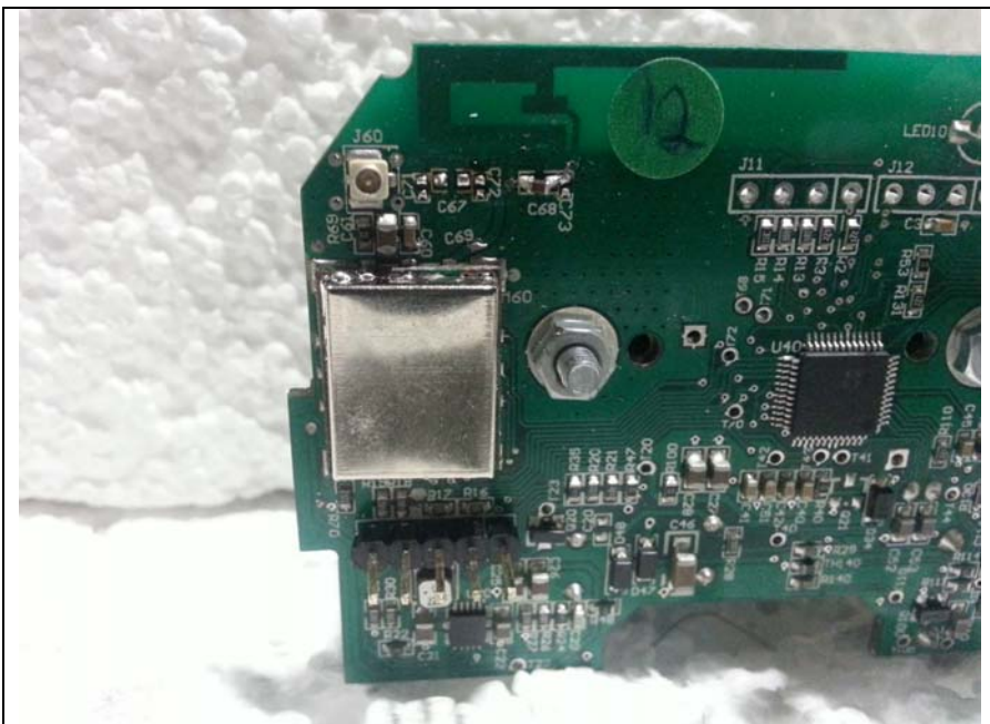
Fig 8 Close up of the module on the host
