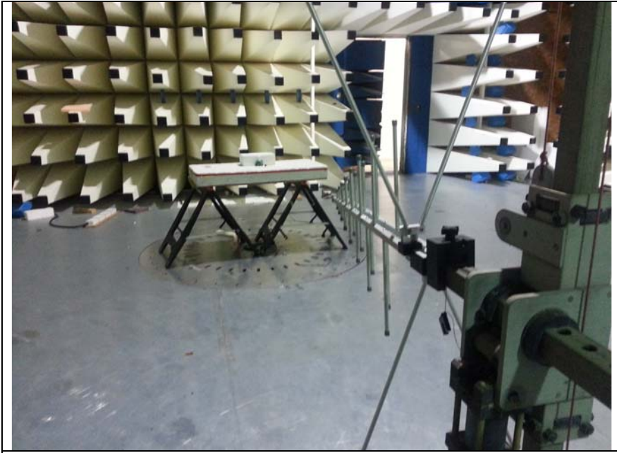
Fig 1 Test setup Rad Emission
