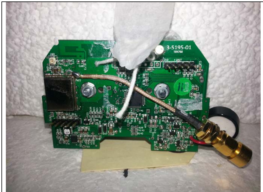
Fig 5 Test setup Radiated Emissions Module port Terminated
