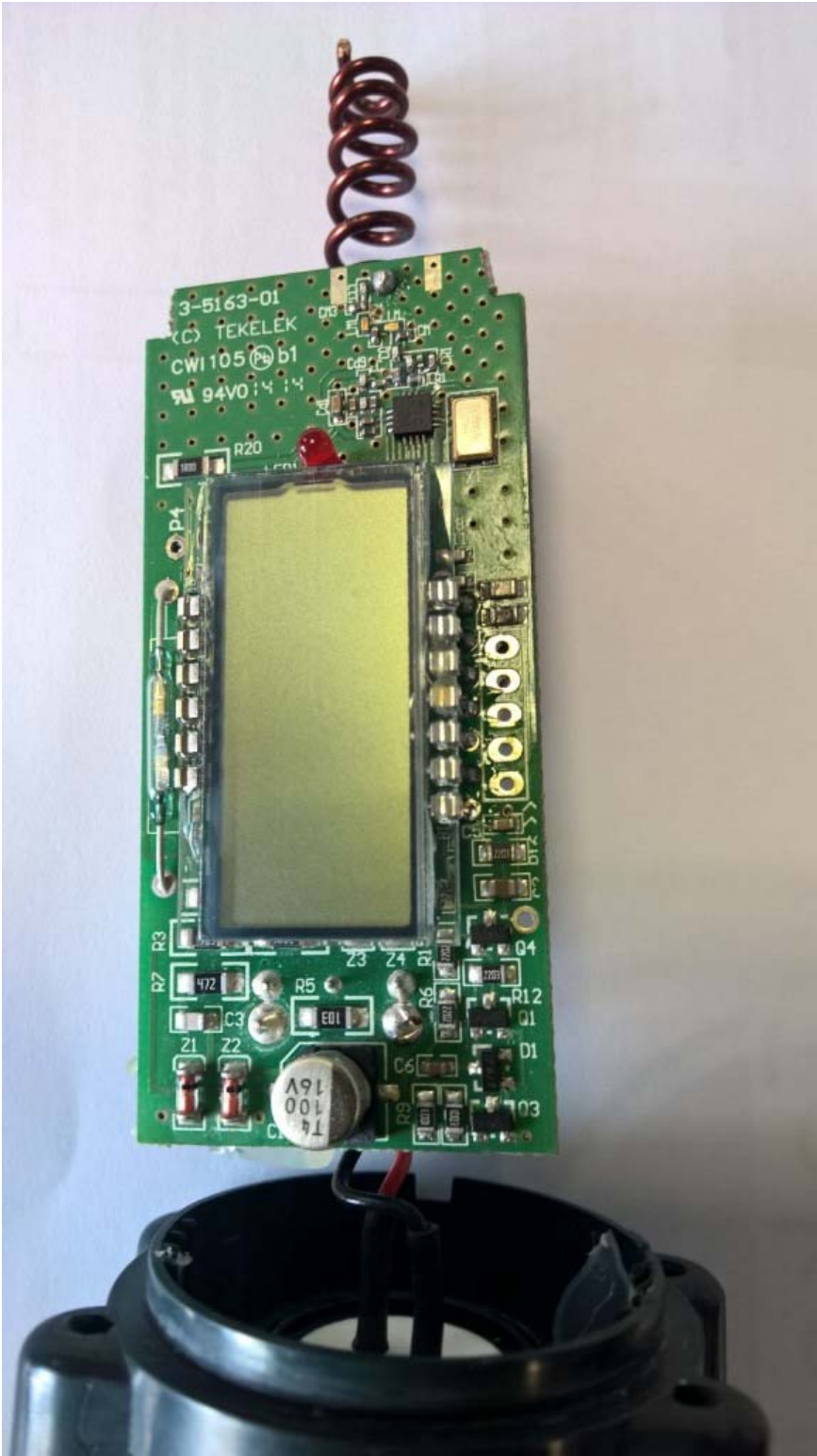
Visual PCB Top side (this has an LCD display).
