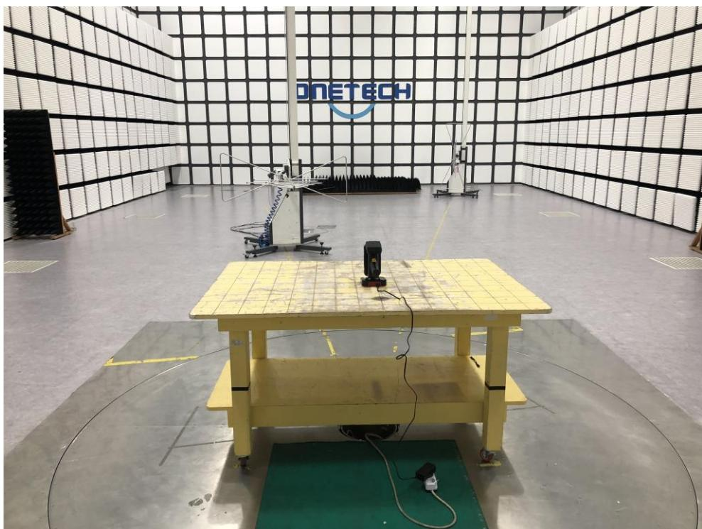
**- Radiated Emission Test (RFID mode)**
