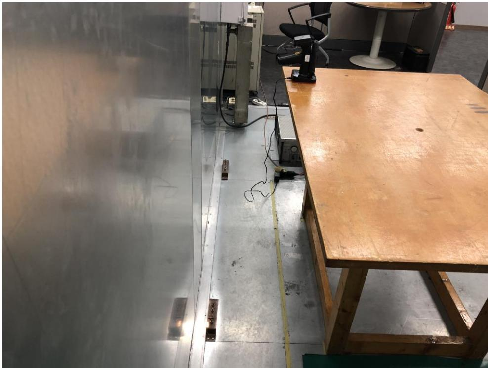
**- Radiated Emission Test (Charging mode)**
