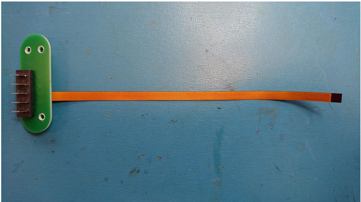
Battery connector flexible circuit 1166B TSL01941
