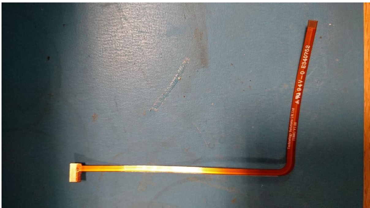
Barcode connection flexible circuit 1166G TSL01951
