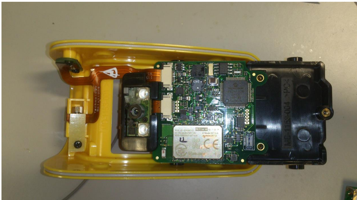
RFID board removed, chassis moved to show flex circuits
