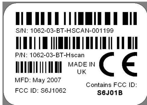
The ID label is 22mm × 31mm. It is fixed behind a window in the main product label which is printed on 0.125mm velvet polycarbonate with a 3M 468MP adhesive backing or equivalent.
