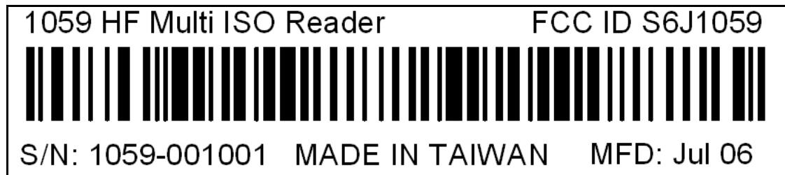
The ID label is 1.8" × 0.4". It is fixed behind a window in the main product label which is printed on 0.125mm velvet polycarbonate with a 3M 468MP adhesive backing or equivalent.
