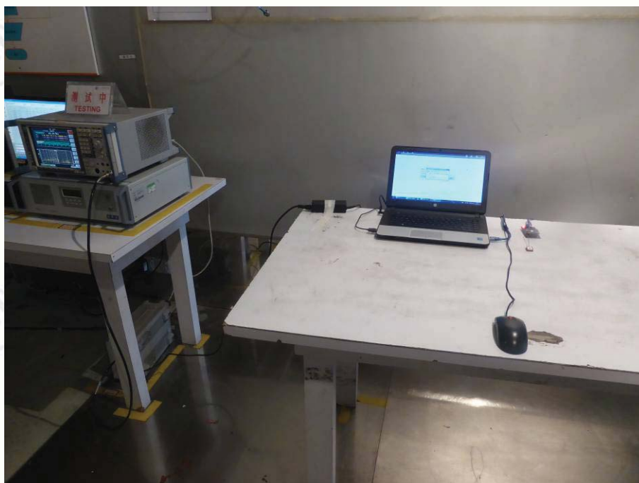
TEST SETUP OF CONDUCTED EMISSION
