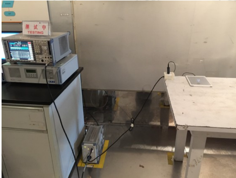
Conducted emission Test Setup
