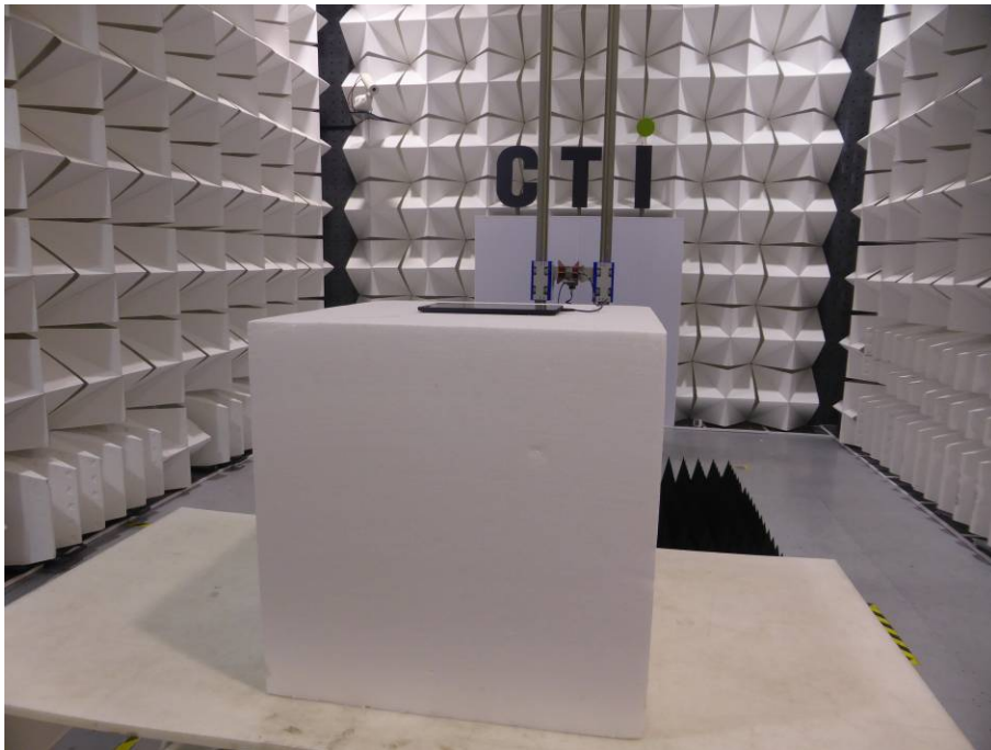
Radiated spurious emission Test Setup-2(Above 1GHz)
