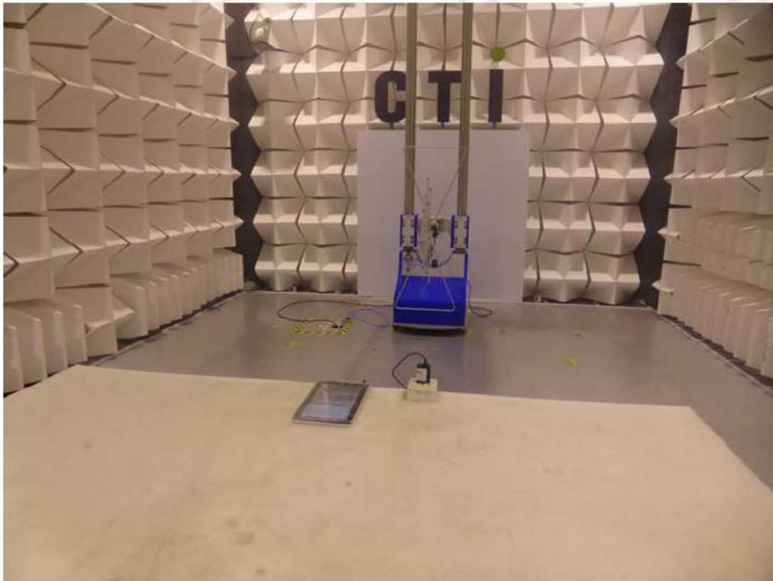
Radiated spurious emission Test Setup-1(Below 1GHz)
