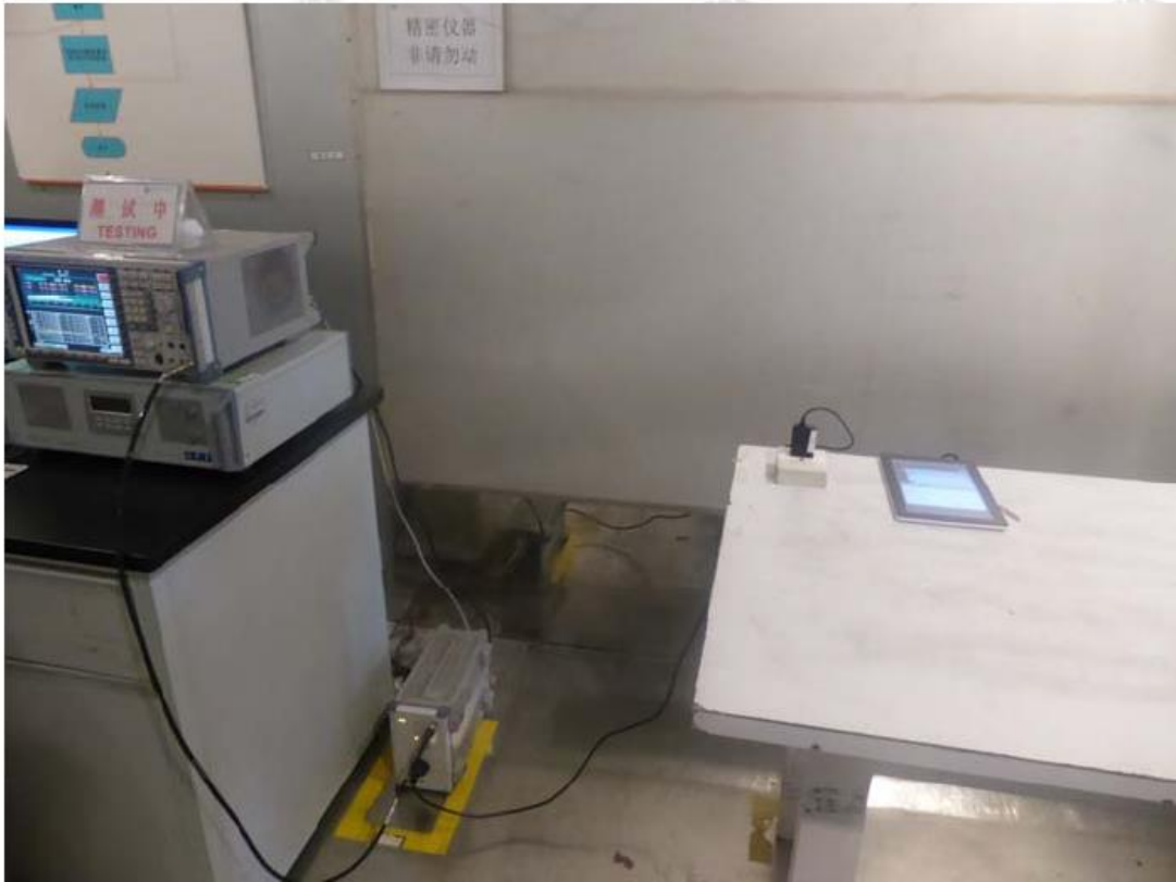
Conducted emission Test Setup
