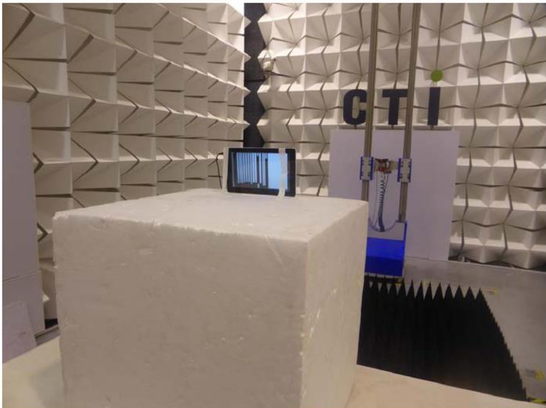
Radiated spurious emission Test Setup-2(Above 1GHz)
