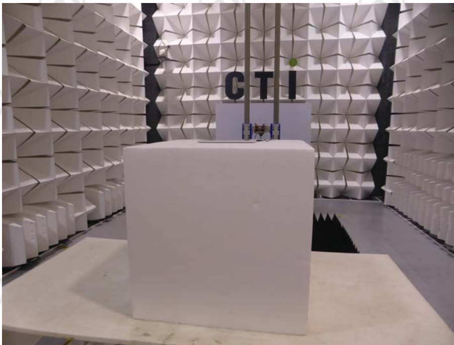
Radiated spurious emission Test Setup-2 (Above 1GHz)
