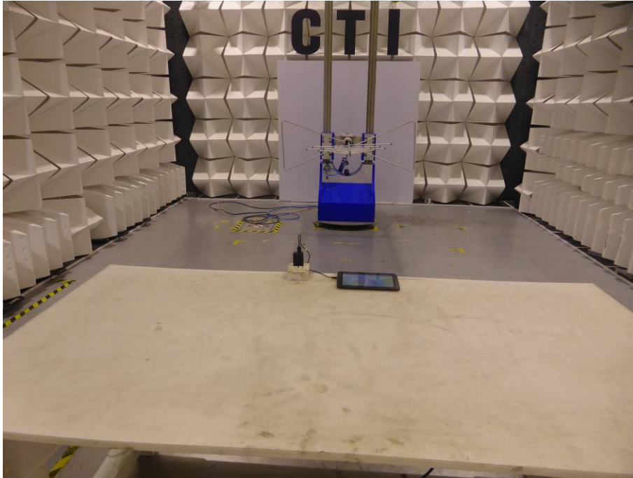
Radiated spurious emission Test Setup-1(Below 1GHz)
