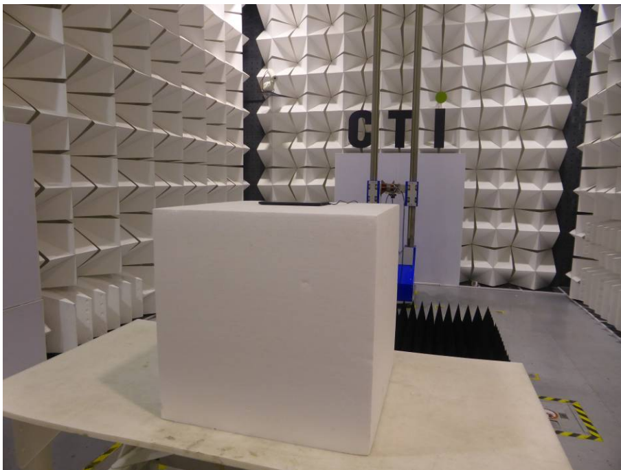
Radiated spurious emission Test Setup-2(Above 1GHz)
