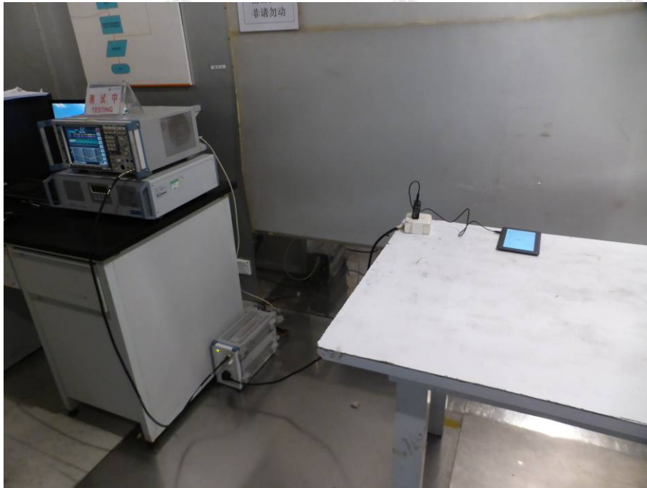
Conducted emission Test Setup
