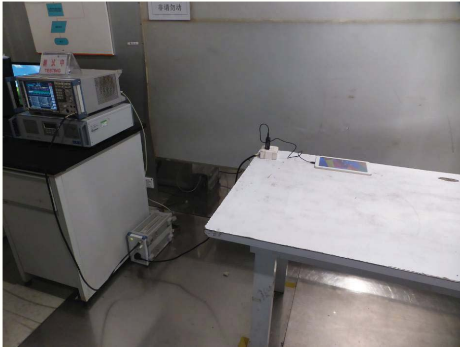
Conducted emission Test Setup
