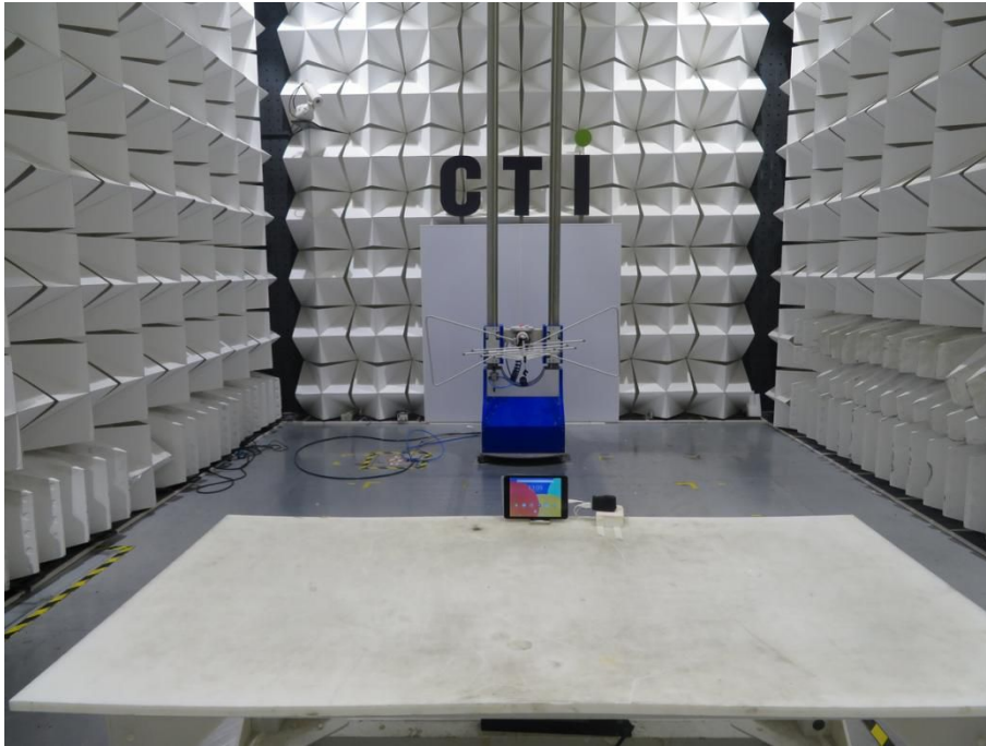
Radiated spurious emission Test Setup-1 (Below 1GHz)
