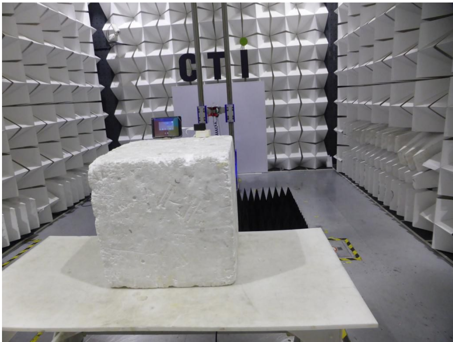
Radiated spurious emission Test Setup-2 (Above 1GHz)
