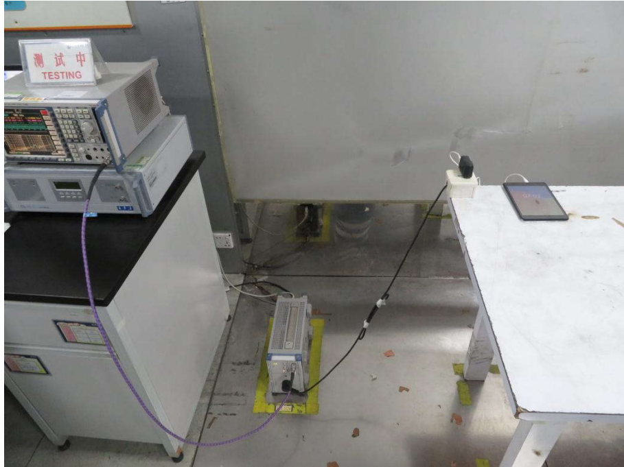
Conducted Emissions Test Setup
