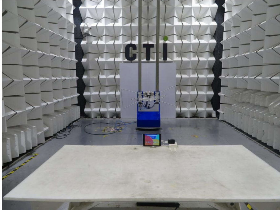
Radiated spurious emission Test Setup-1(Below 1GHz)
