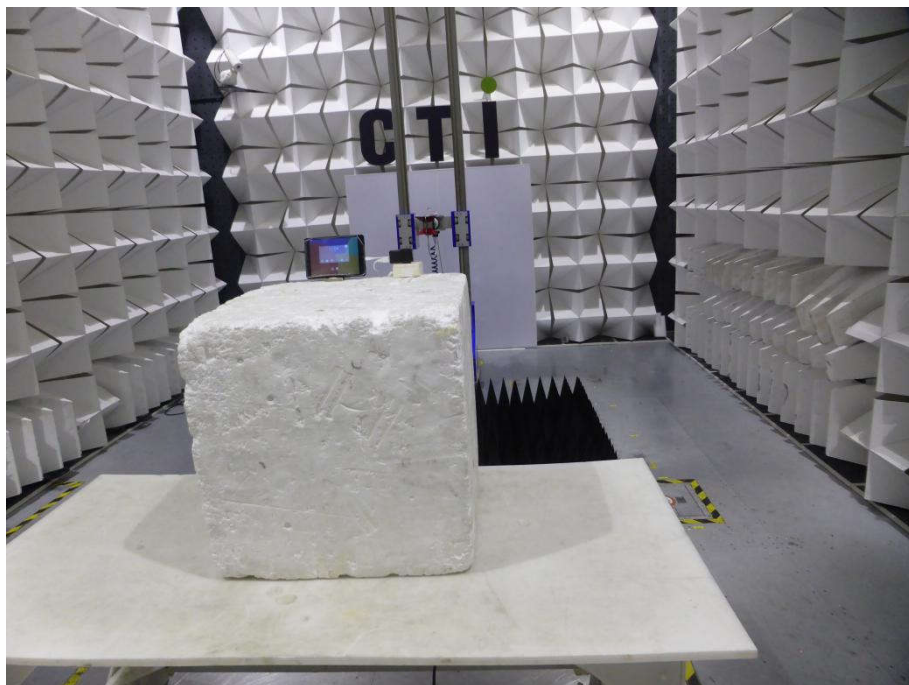
Radiated spurious emission Test Setup-2(Above 1GHz)
