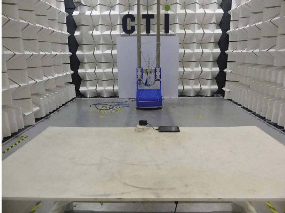
Radiated spurious emission Test Setup-1(Below 1GHz)
