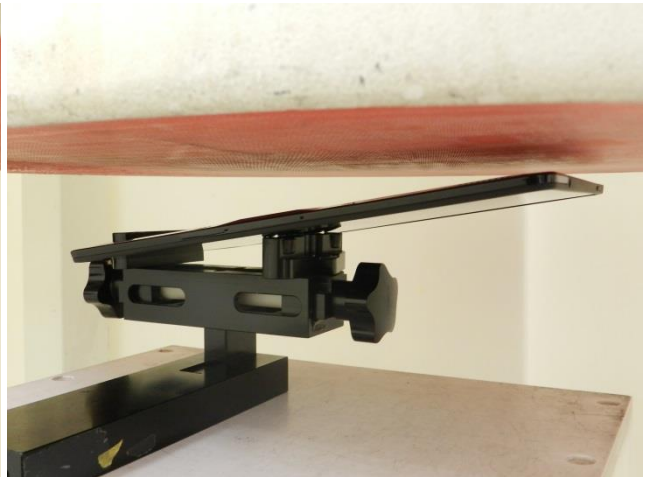
Bottom - Slant of Edge 2, Test Separation 1.3 cm
