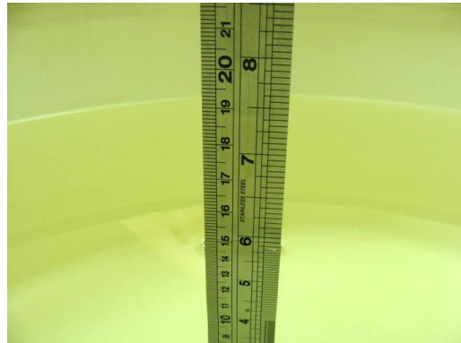
Fig 6.2 Photo of Liquid Height for Body SAR
