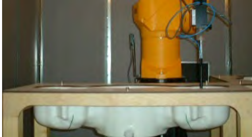
Figure 2.6 SAM Twin Phantom
