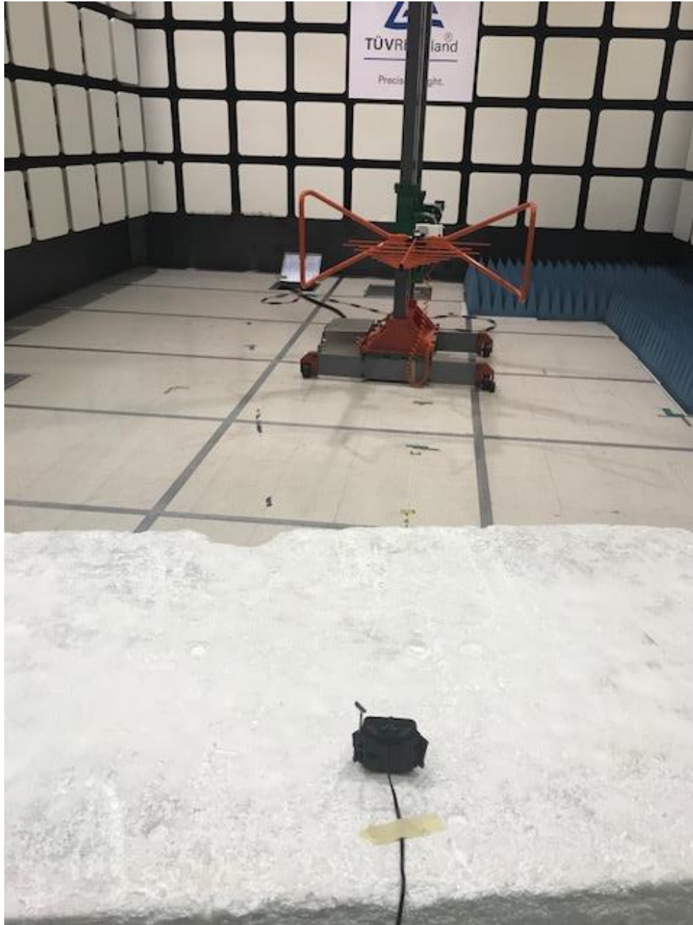
Radiated Emissions Setup 30 to 1000 MHz rear
