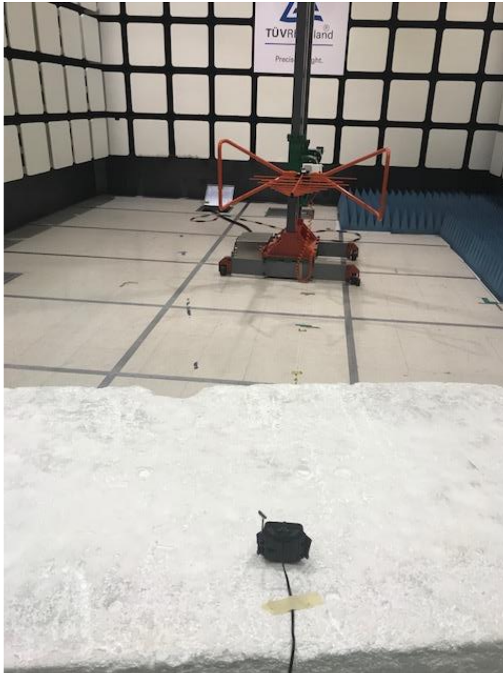
Radiated Emissions Setup 30 to 1000 MHz rear
