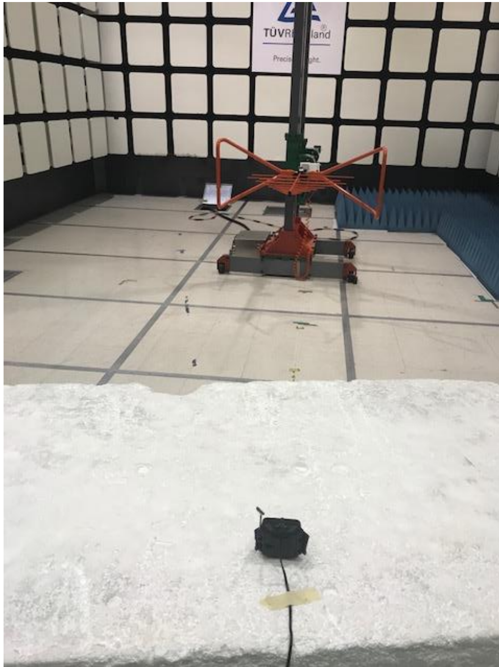
Radiated Emissions Setup 30 to 1000 MHz rear
