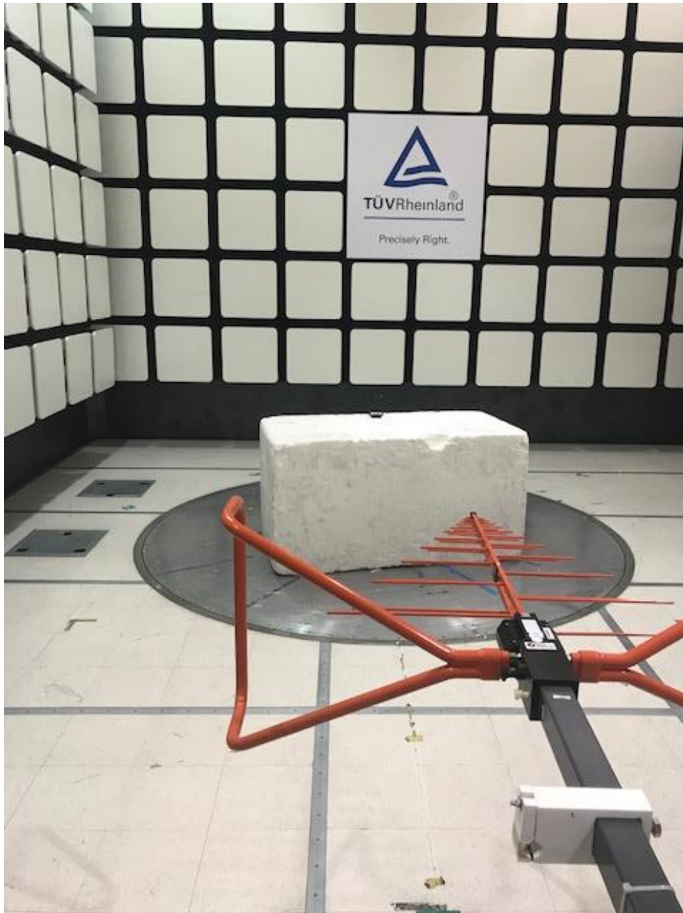
Figure 1 - Radiated Emissions Setup 30 - 1000 MHz - Front
