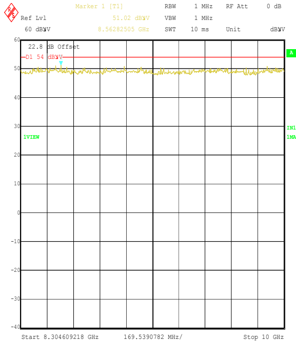
Title: 47271JD01 Sattelite Tracking Of People FCC Part 24 Comment A: Radiated Spurious Emissions RX Mode Date: 11.MAY.2005 20:41:37
