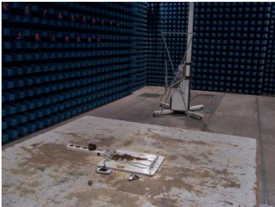
**4. Radiated Emission Test, USB Mode**
