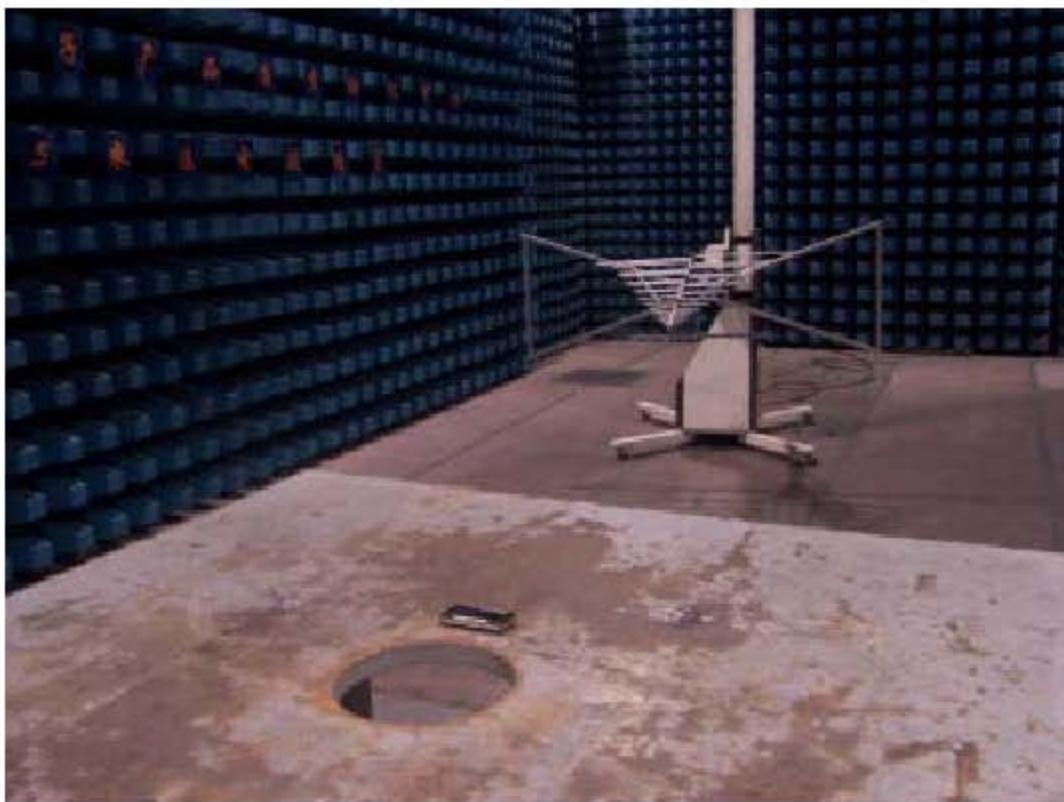
**4. Radiated Emission Test (above 1 GHz)**
