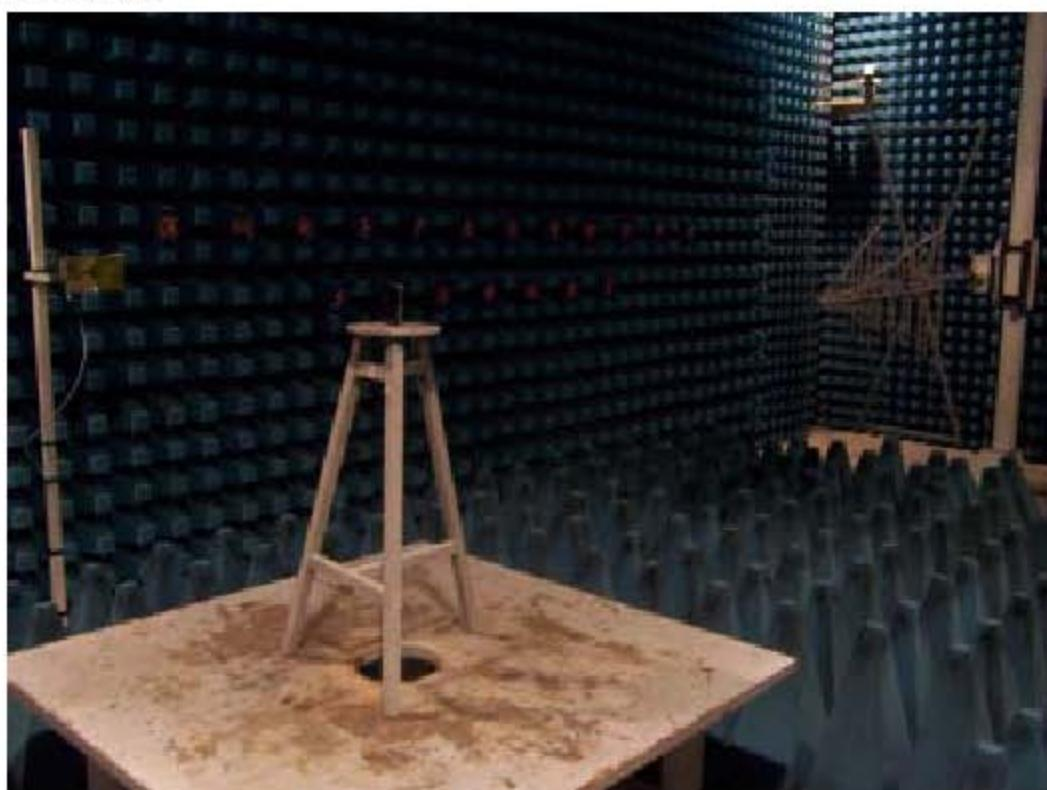
**3. Radiated RF Test (9kHz~30MHz)**
