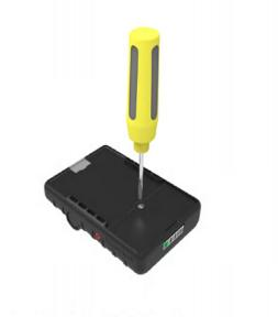
4. Pull the battery cover and remove it from the personnel RTLS Tag enclosure.
