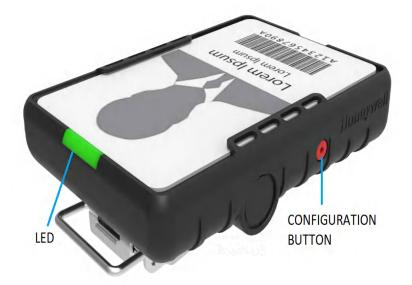
RTLS Tag will join the OneWireless user interface (ISA100 network). For more information, see section Description of RTLS Tag parameters
