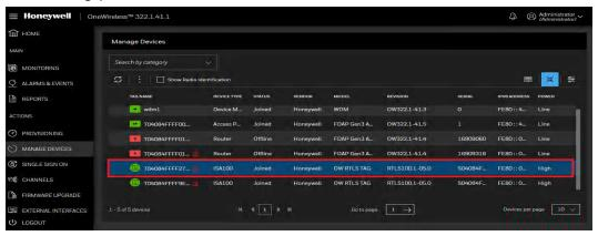
4. RTLS Tag can be identified with the icon as shown below:
