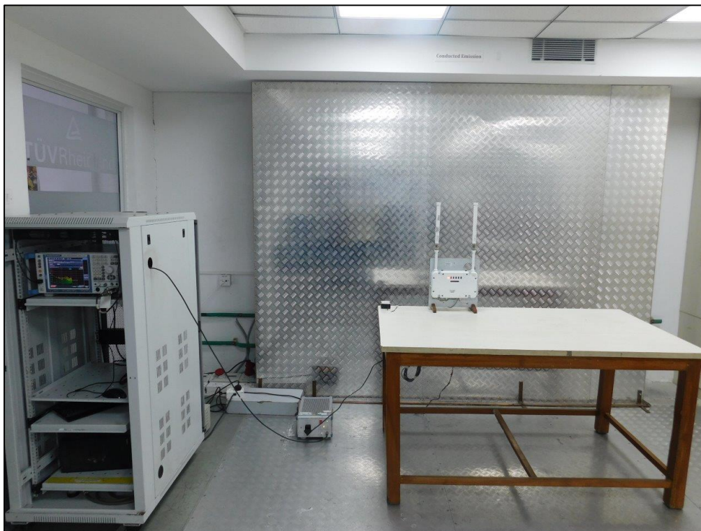
Conducted emission test setup
