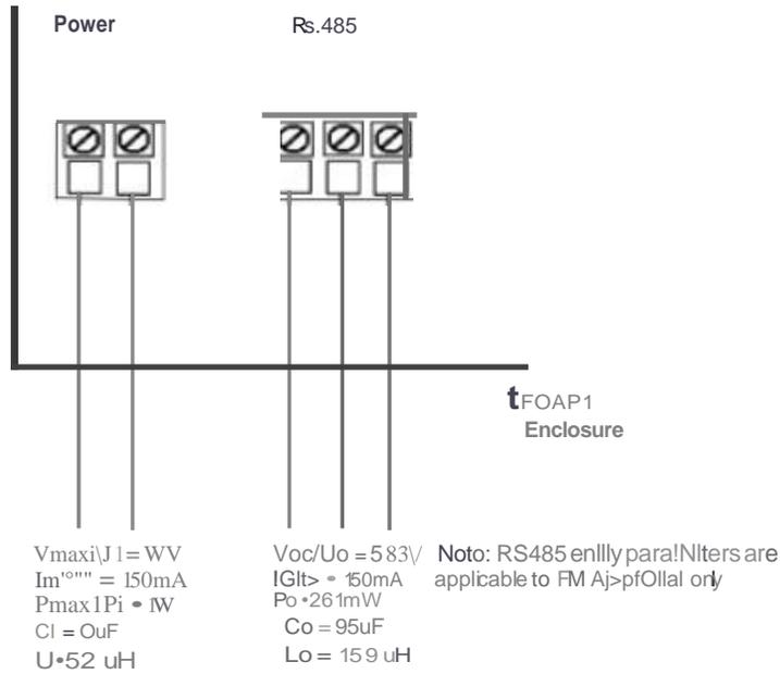
**Note:** Ethernet connections are not allowed in intrinsic safety installations
