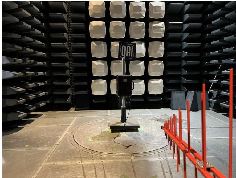
Figure 1: Radiated Emissions 30MHz- 1GHz
