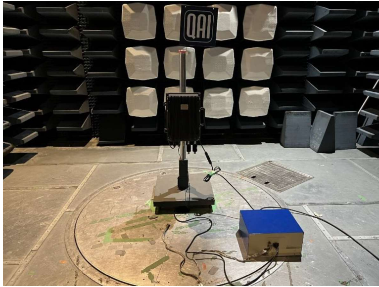
Figure 3: Conducted Emissions AC Main.
