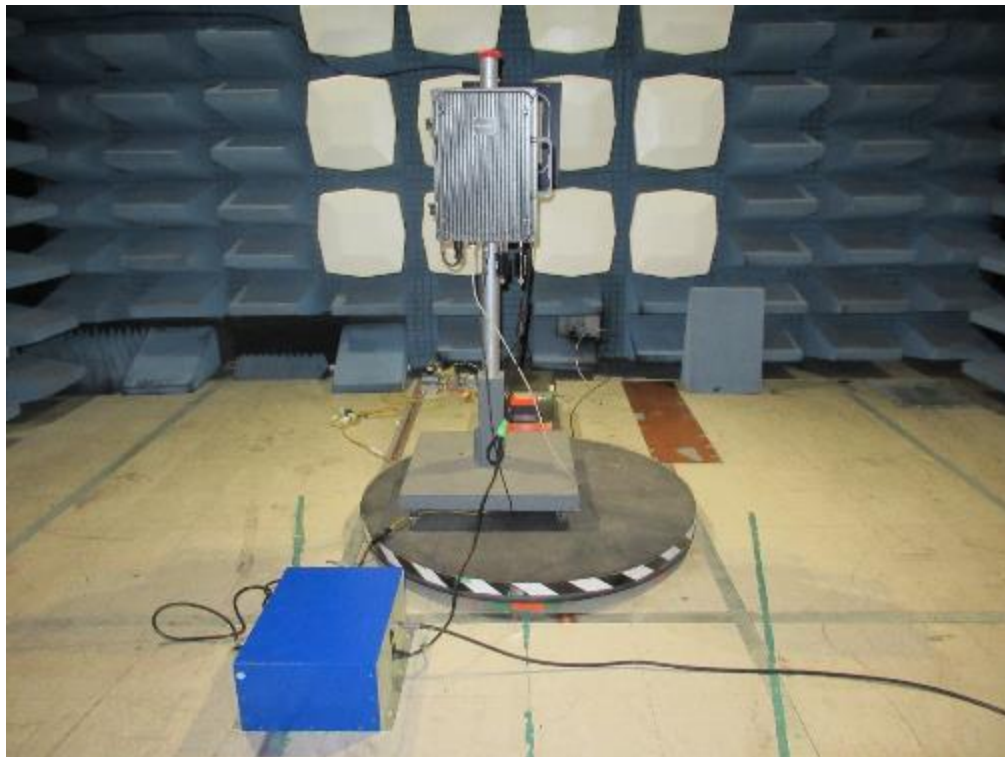
Figure 164: Radiated Emissions: 30 MHz – 1 GHz Measurement Setup
