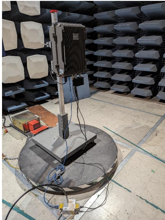
Figure 82: Conducted Emissions: Telecom Measurement Setup
